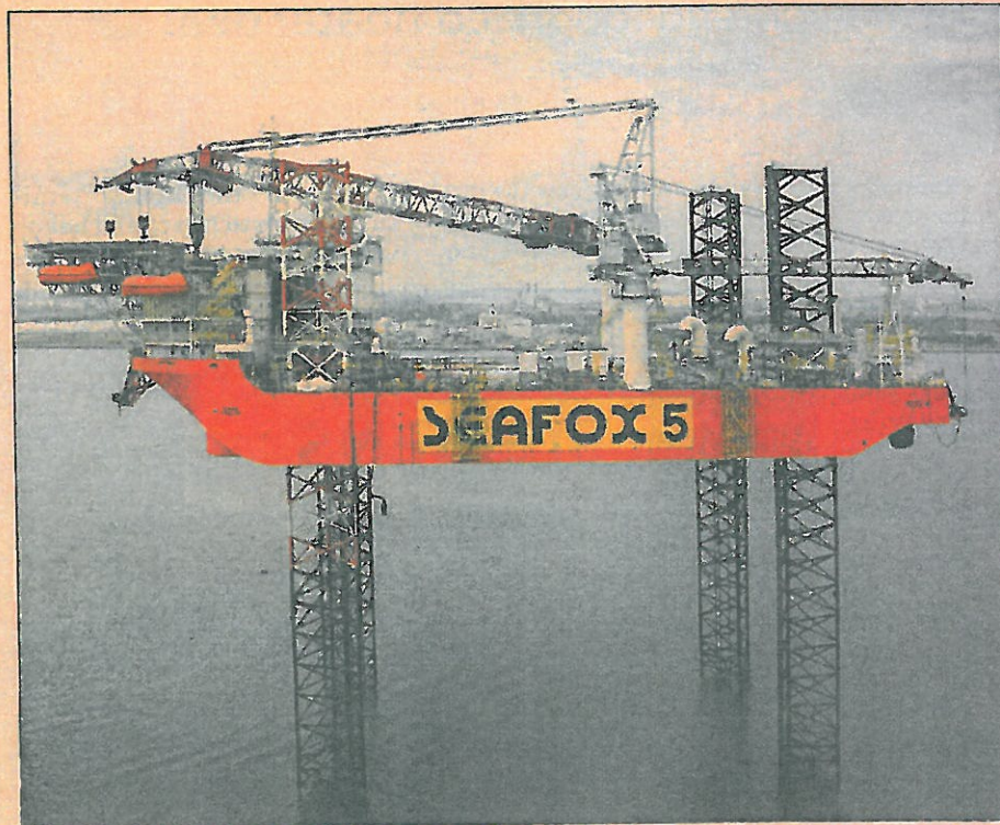
Sea trials: the multi-purpose offshore installation jack-up Seafox 5
