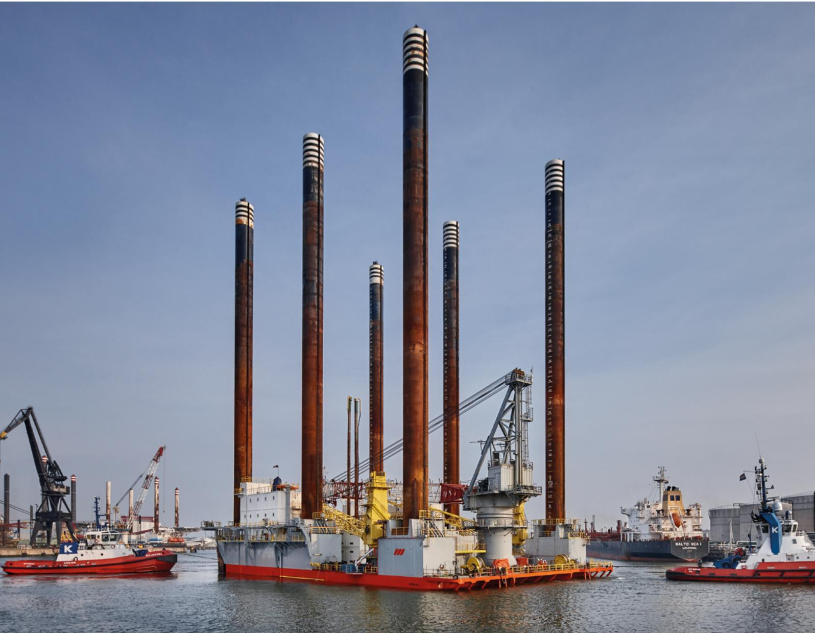
MAIN CRANE CAPACITY 300 t | ACCOMMODATION 153 POB | MAX WATER DEPTH 45 m | DECK SPACE 900 m<sup>2</sup>
